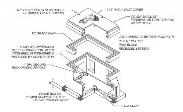
\* MIN EXCAVATION 36" x 72" x DEPTH OF BOX
