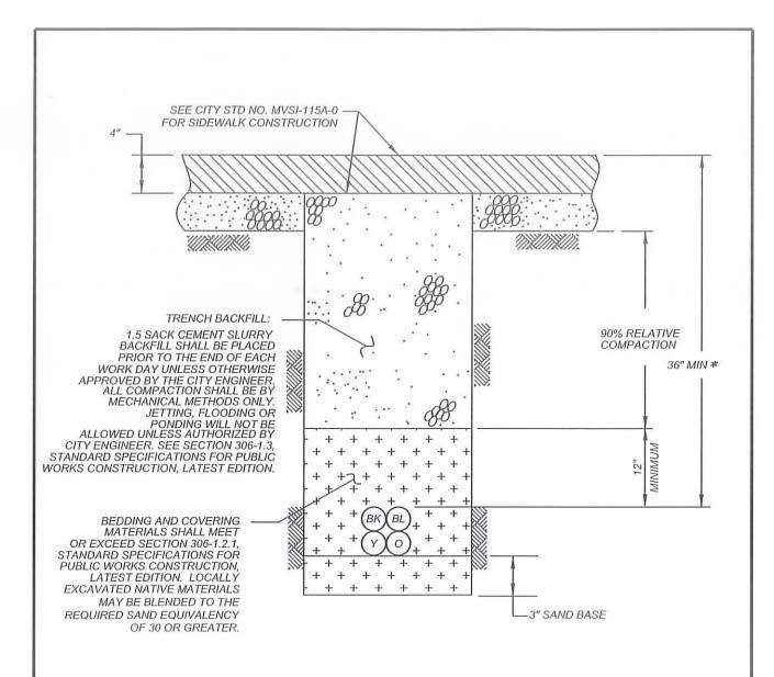
\* 36" MIN FOR TRUNK AND DISTRIBUTION CONDUIT SYSTEM AND 18" MIN FOR SERVICE LATERAL CONDUIT SYSTEM.
