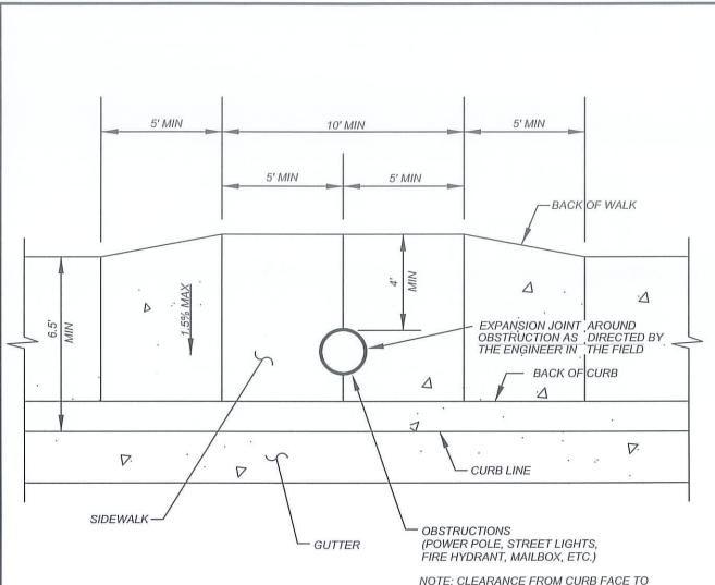
NOTE: CLEARANCE FROM CURB FACE TO FACE OF POLE SHALL BE 18" MINIMUM.
